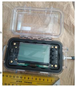
buttons to adjust the device settings, and to calibrate it. Inside the cave there is a mini-B USB socket that is used to recharge the device battery as well as to connect it to a PC to downlad files. A mini-B USB connector is not very common nowadays - it is an old connector that you might find at home if you have an old digital camera. The BRIC4 can be charged from the PC. While charging the main screen shows the battery charge with a flickering percent symbol.
